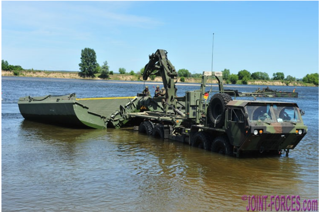
A M1977A2 HEMTT Common Bridge Transporter recovers a M17 Interior Bay of the Improved Ribbon Bridge at end of a bridging operation [© Carl Schulze]
